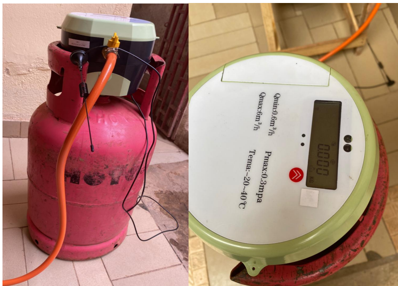
Figure 13 : Gas Device on Bottle: This is image show the bottle with the gas metering device.
