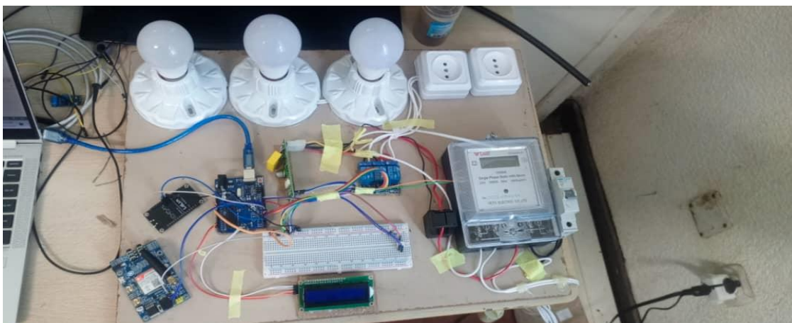
Figure 4. 1: Connection of the system.
