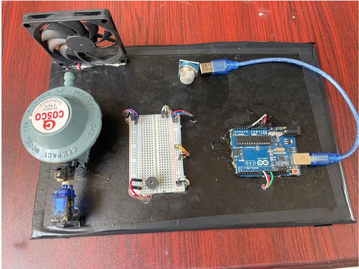
Figure 14: The assembled system components
