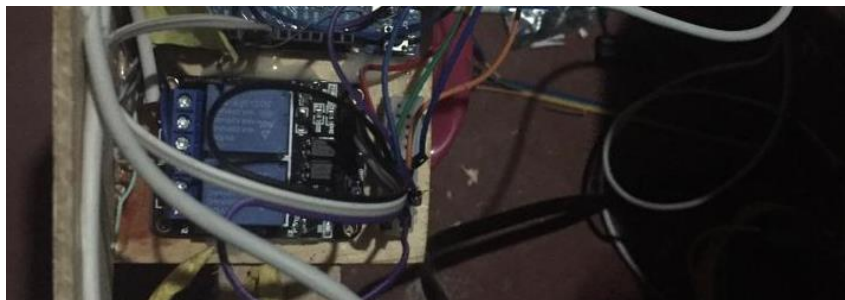
Figure 13: Relay in circuit
