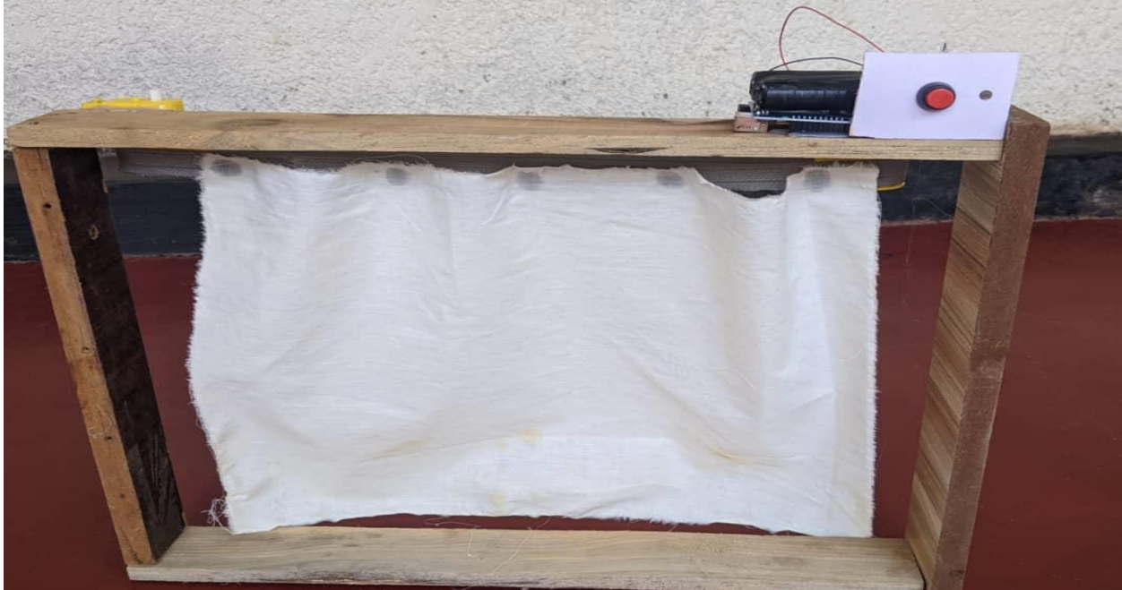
Figure 19: Curtain is closed using LDR.
