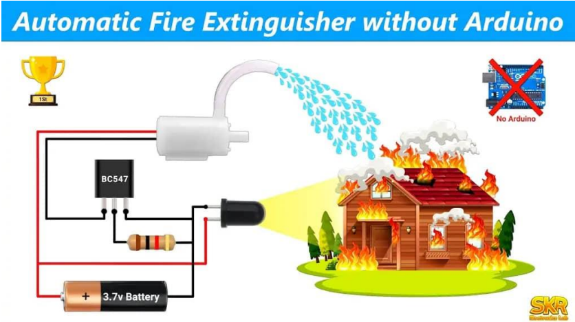
Figure 1 Automatic fire extinguisher without arduino
