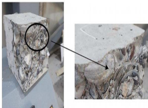
Figure 3.16: Clumping of long fibers inside the concrete.
