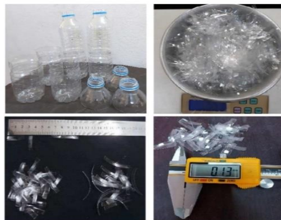
Figure 3.10: PET waste fibers used in this study.
