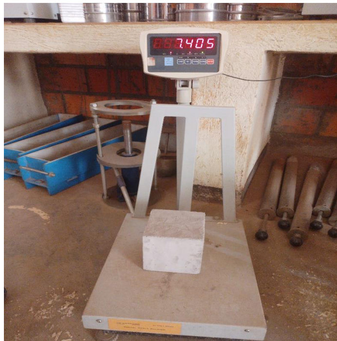
Figure 4.6: Dry weight of a concrete cube
