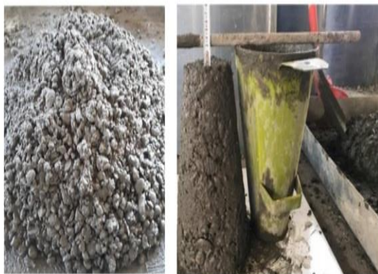
Figure 3.12: Slump test and concrete flow
