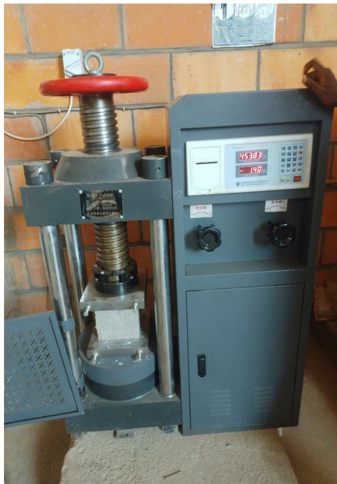
Figure 4.7: Sample in a compression machine after being crushed
