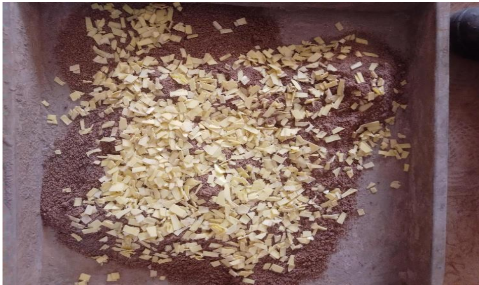
Figure 4.2: Plastic flakes on fine aggregates
