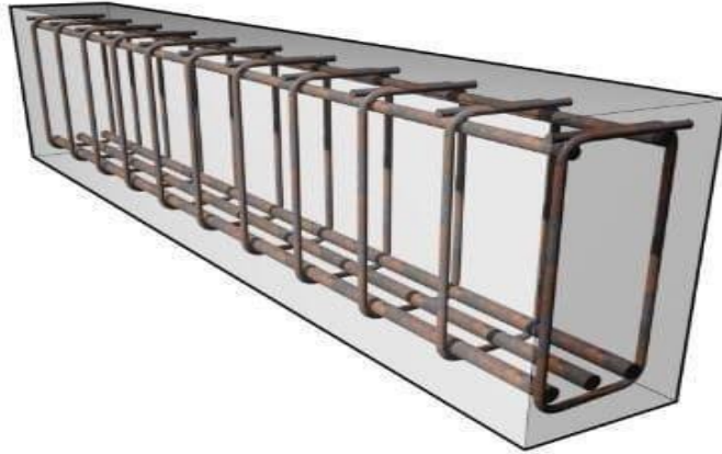
Figure 2.1 :Reinforced concrete beam (Mosley, 1990)
